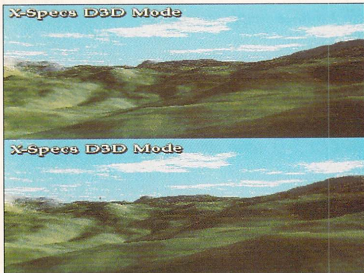
Figure 1. The "over-under" format of an X-Specs D3D stereo image. Left and right views are stacked in a single interlaced image. The views were created in Scenery Animator.
